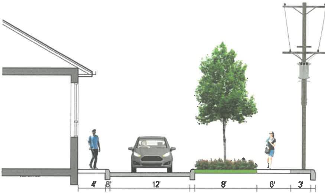
Figure 3. Cross-section of 35-foot commercial setback
